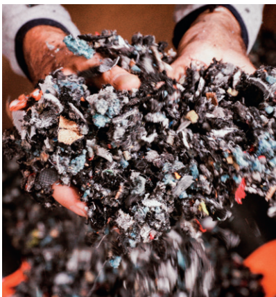
(4) Liners' crashing flakes output
