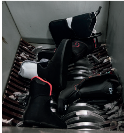
(2) Liner mechanical crashing phase
